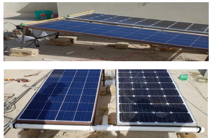
Figure 1 Lower side view of the solar panel installed with piping
